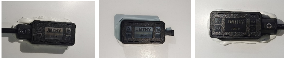
Fig. 3: View of junction box of module type ERA Pro-72HC580M
